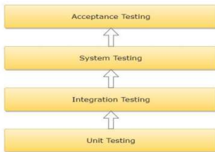
Fig 6.3 Levels of Testing
